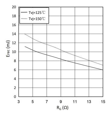
switching losses Diode, Inverter (typical)
